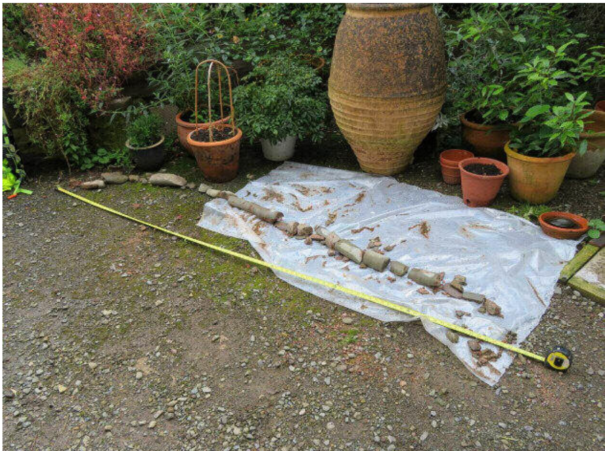
Photograph 25: Core P1 removed and laid out
